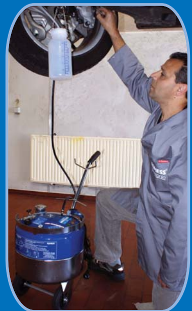
The "Romessage" shows how ROMESS service equipment can be used profitably in the workshop; top leak detector USM 20128; below brake service with the S 15.
