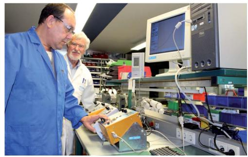
To ensure that they operate reliably and with high precision, the AQUA Series brake fluid testers are carefully adjusted during production.
